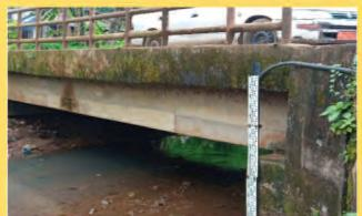
View of a water level station and the cable connecting the submerged pressure sensor module to the central unit installed on the bank.
